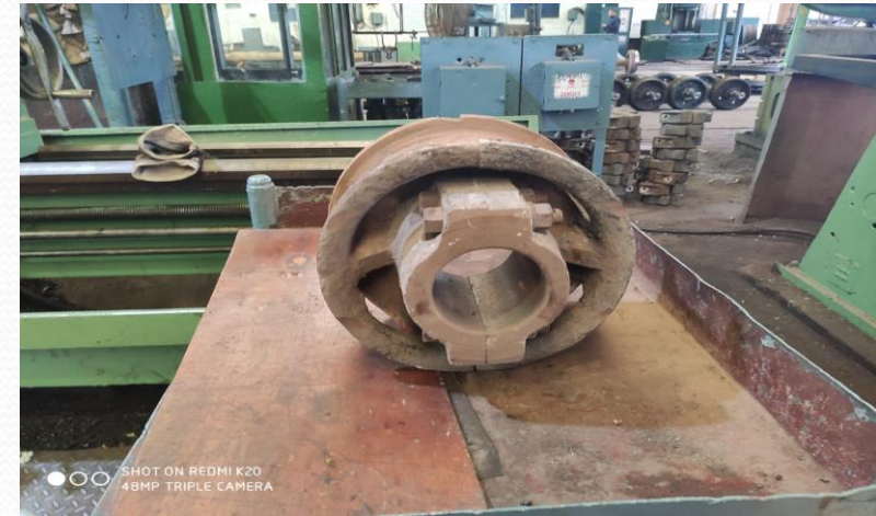
Existing Cast Iron Pulley (wt - 52 kg.)
