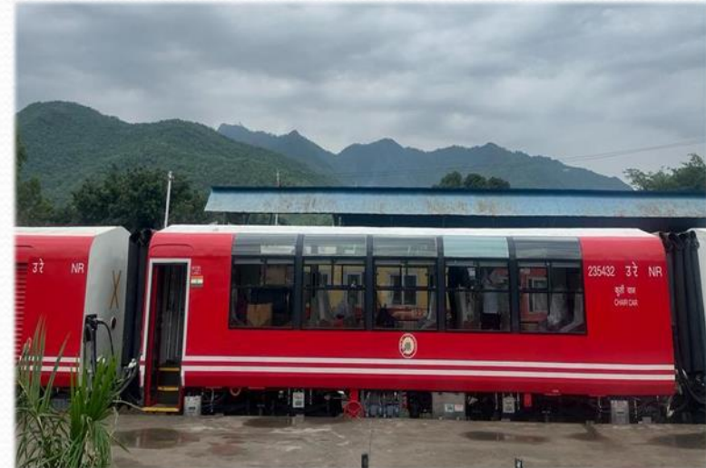
Fully Fabricated SS Shell NG coach with Modified bogie
