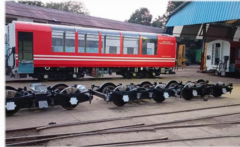
Fully Fabricated SS Shell NG coach with Modified bogie
