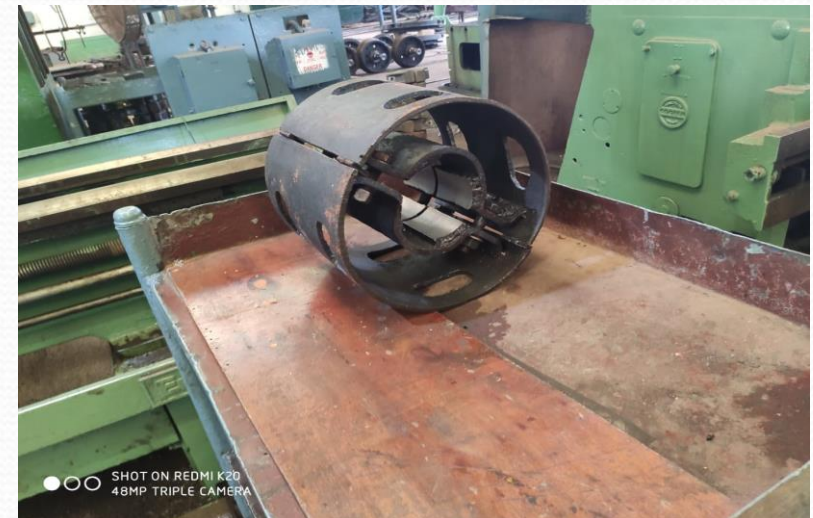
Newly developed fabricated Pulley (wt - 28.5 kg.)
